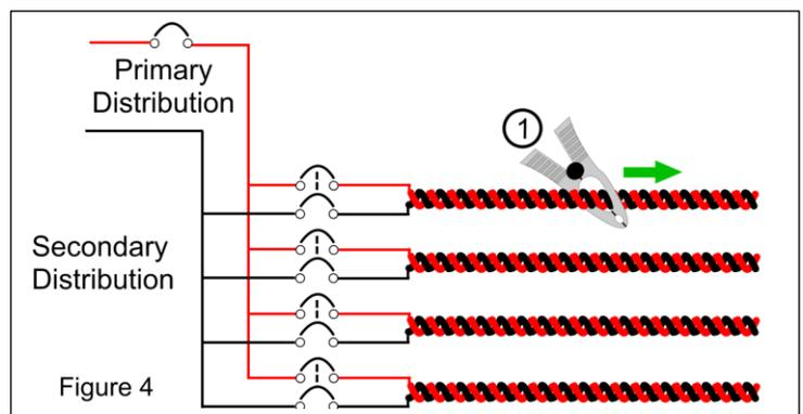
If the distance from the signal generator to potential ground fault is so far that the signal strength is falling off, it is possible to move the signal generator further in to the distribution system and reset the reference using Clamp 1, which should be the clamp that was used to set the initial reference.
