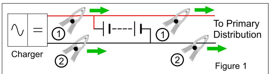
negative cable depending on which was identified as being the source of the ground fault. If the reference level is not stable, then it will be necessary to use the second current clamp which should be placed on the opposite polarity cable. The green arrow on the cable clamps should be pointing towards the battery and primary distribution, away from the charger.
